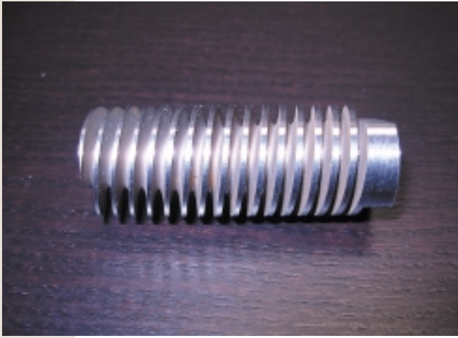
Illustration #3 Turn while Burn technology makes it possible to machine this helix screw on a wire EDM.
