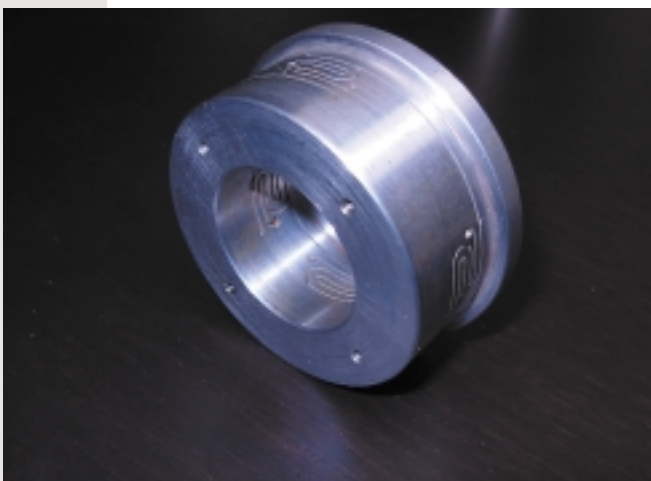
Illustration #5 The small, complicated slots in this squeeze film damper were produced almost exclusively through B-axis movement on a wire EDM.
